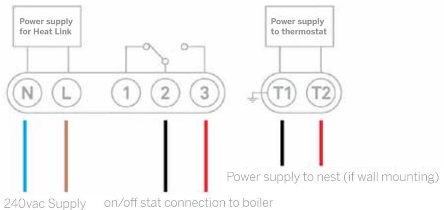
\* Charging stand required if nest is not to be powered using T1 and T2 connections (powered via USB cable supplied with charging stand)
